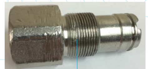
Damage to threads on SDX III Nozzle
